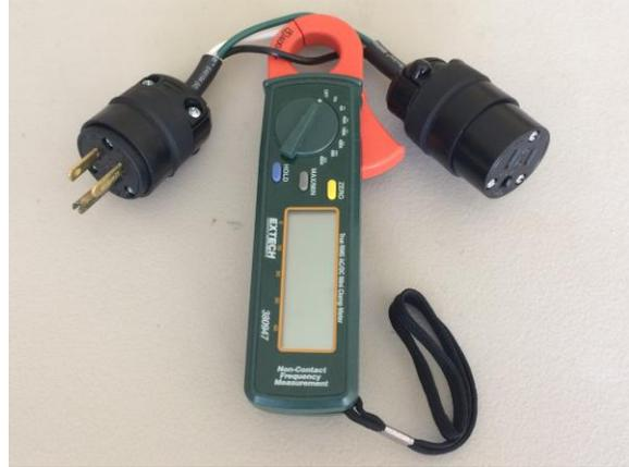
You may have a different method or location to make this measurement. Just be sure the measurements are made at a location that includes all loads on the generator.
