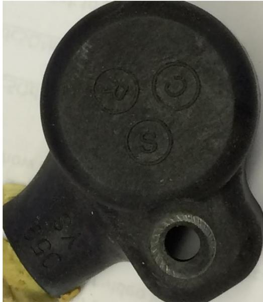
Some caps have the windings marked on the top as shown while others have markings inside the cap. Some compressors also stamp a letter on the compressor housing to indicate the connections.
