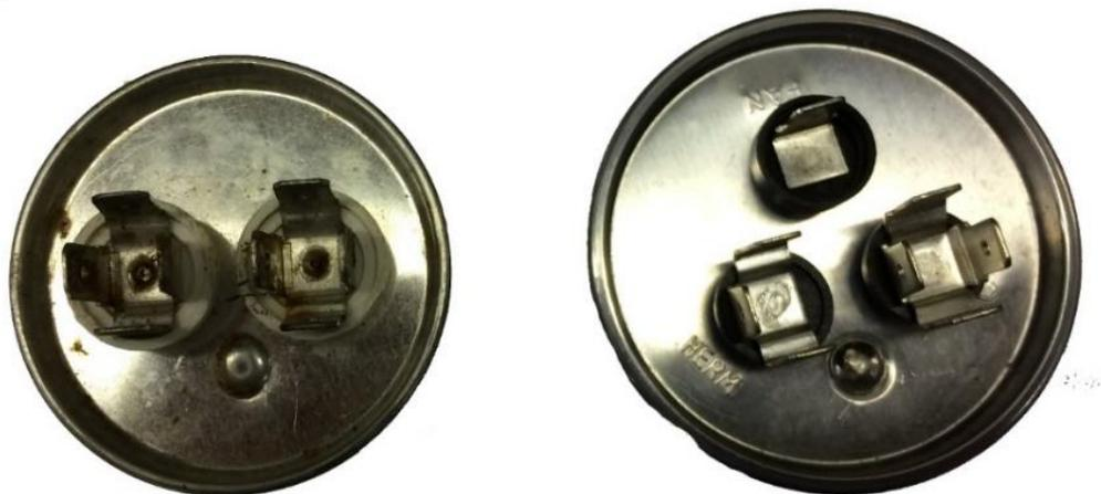
Notice that on the capacitors there are provisions for multiple connections. These connections are organized into groups of one to four connections. The “S” wire followed at the end of the previous step should connect to the HERM terminal on the three-terminal capacitor and one of the two terminals on the two-terminal capacitor. This terminal group on two terminal capacitors can be considered the HERM terminal group. The Orange wire from EasyStart must connect to HERM terminal group.
