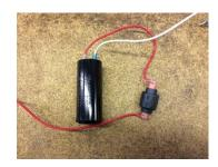
9. Connect the orange wire from EasyStart to the same terminal group on the run capacitor as the red wire connected to the compressor start winding. This terminal is often labeled HERM on top of the capacitor.
