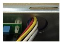
6. Install the split plastic bushing provided in the kit. The split allows it to slide over the existing wires without having to disconnect them. Snap it into place in the existing hole. Once the bushing is in place, route the wires from EasyStart through the hole.
